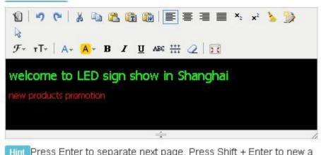
Hint Press Enter to separate next page, Press Shift + Enter to new a line. Define the following string instead of the value of sensors in terminal: %c is celcius, %f is fahrenhite, %h is humidity, (%c1 %f1) or (%c2 %f2) round to 1 or 2 digit(s) after the decimal point
