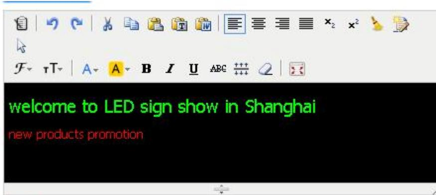
**Hint** Press Enter to separate next page, Press Shift + Enter to new a line. Define the following string instead of the value of sensors in terminal: %c is celcius, %f is fahrenheit, %h is humidity, (%c1 %f1) or (%c2 %f2) round to 1 or 2 digit(s) after the decimal point
